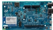
Figure 2. Intel Edison System on a Chip plugged on an Arduino Board [47]
